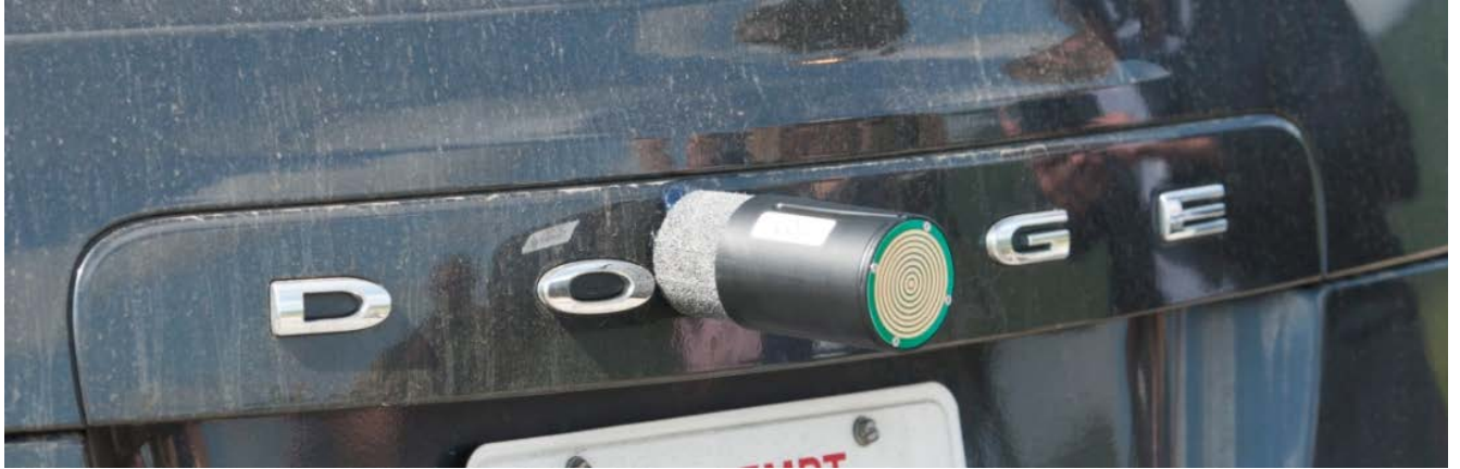
The STAR CHASE Projectile after it has struck and adhered to the back of a vehicle.
